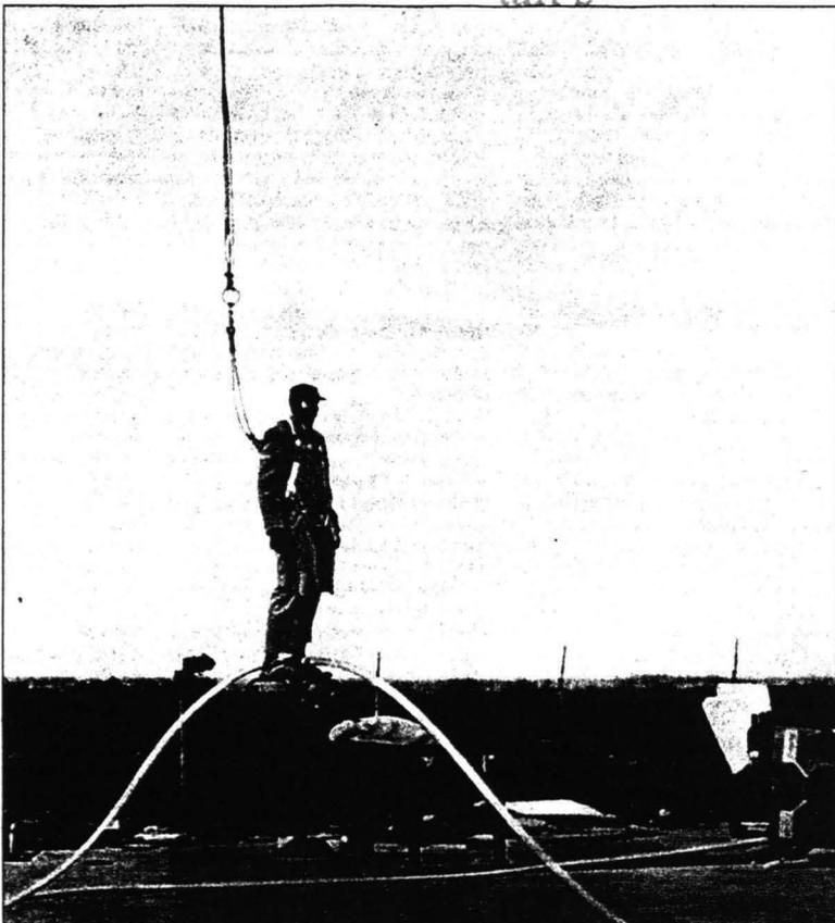
This photo, published July 9, 1955, on the cover of the Illustrated London News, shows Paul Hill hovering. Hill tapped a supply of 200 psi compressed air, normally used to operate a supersonic wind tunnel, and connected it with fire hoses to a special nozzle. Courtesy of "Unconventional Flying Objects"
